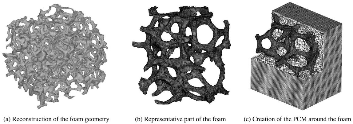
Figure 2: Meshing of the PCM embedded inside open cell foam
