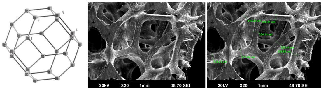
Figure 1: Tetrakaidecahedron and measurement of the foam pore size
