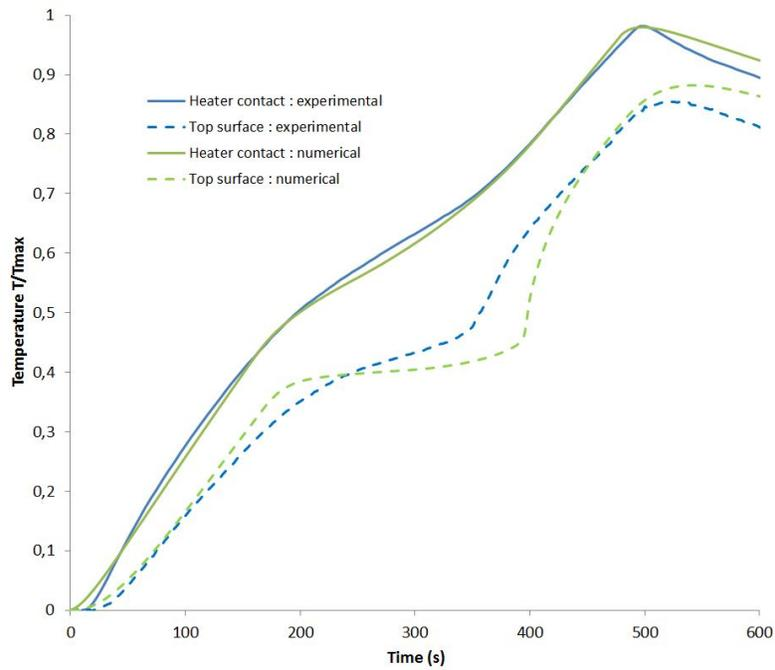
Figure 3: Experimental and numerical comparison for PCM embedded inside open cell metal foam
